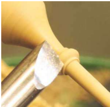
▲ Pic.23 The gun barrel bead is a very traditional design and is in keeping with the project. The tiny fillet on either side helps to define the detail
